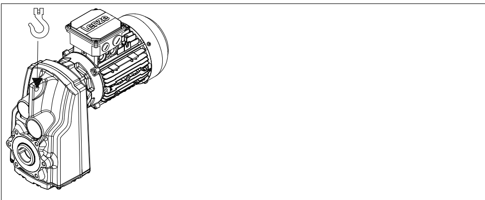
Fig. 2 Ear for transporting the complete drive system
