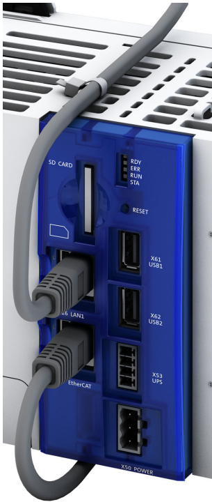
Fig. 1: Installation and fixing of the network cables
